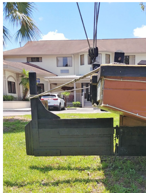
Note the flat bottom, large leeboard, and rope-controlled tiller all made from wood.
